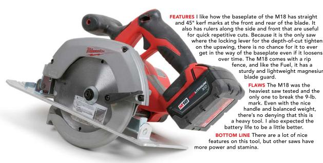
FEATURES I like how the baseplate of the M18 has straight and 45° kerf marks at the front and rear of the blade. It also has rulers along the side and front that are useful for quick repetitive cuts. Because it is the only saw where the locking lever for the depth-of-cut tightens on the upswing, there is no chance for it to ever
