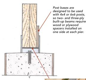
If the beam needs to be shimmed to get it level, use shim stock that won't compress under load and won't deteriorate from rot or rust. Galvanized metal tie plates (sometimes called strap ties) are a good option and can be bent in half for extra thickness.
