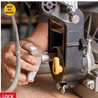
Mounted on the saw arm and facing the user, the Bosch's bevel lock can be reached without a stretch. The bevel locks on the other saws, such as the DeWalt (above), are at the very back. To change the setting, you need to reach around behind the saw arm, which is less convenient.
