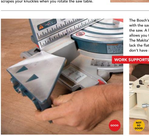
The Bosch's work supports are perfectly aligned with the saw table and fully retract for transporting the saw. A large flat surface on top of the supports allows you to clamp a stop block for repeat cuts. The Makita's supports (below) are options, and they lack the flat surface for a stop. The other saws don't have supports at all.
