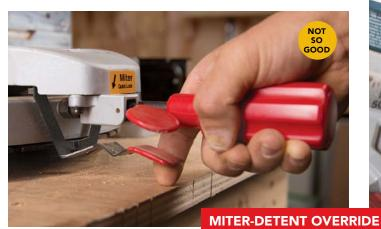
Miter detents stop the saw table at common settings, but it's sometimes necessary to turn off the feature for miters that land close to but not quite at a detent position. The Bosch's detent override is right above the miter lock, where it's easy to use. On other saws, the override is harder to use. On the Craftsman (above), for example, the override scrapes your knuckles when you rotate the saw table.
