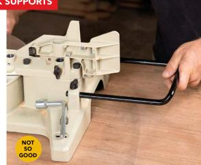
Built with a plastic duct that helps direct dust into the on-board bag, the Bosch saw is 75% effective at dust collection and gets even better when a vacuum is attached. The other saws, such as the Skil (left), have poor dust collection in comparison, even with an attached vacuum.
