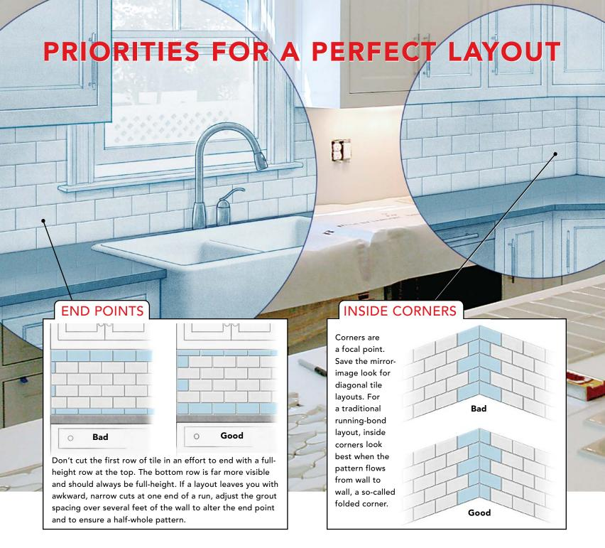
terms of layout or installation, the backsplash becomes a daily eyesore. The good news is that a pleasing layout isn't hard to achieve, and the process of laying up and grouting tile isn't complicated, as long as you plan carefully and work through each step slowly.
