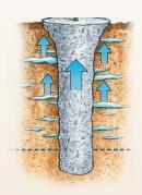
Debris: Rocks, roots, pipes, and other projections that impinge on the straight sides of footings can give purchase for frost to heave or tilt footings. They also leave defects in the footing that can lead to concrete fractures.
