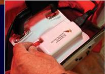
Install the fan. Insert the blowerdoor fan through the elastic hole in the fabric cover. Once it's in place, secure it to the intermediate frame rail with the Velcro strap, and attach the red hose to the air fitting on top of the housing.
