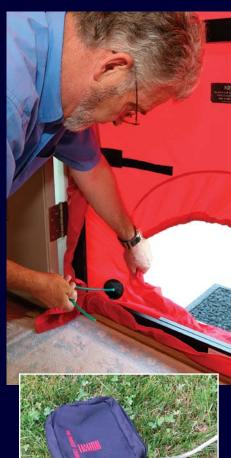
Route the hose. The air hose that measures outside air pressure is routed through a small hole. Putting the open end at least 5 ft. from the fan and inside the unzipped manometer storage bag prevents strong winds from distorting the measurement.
