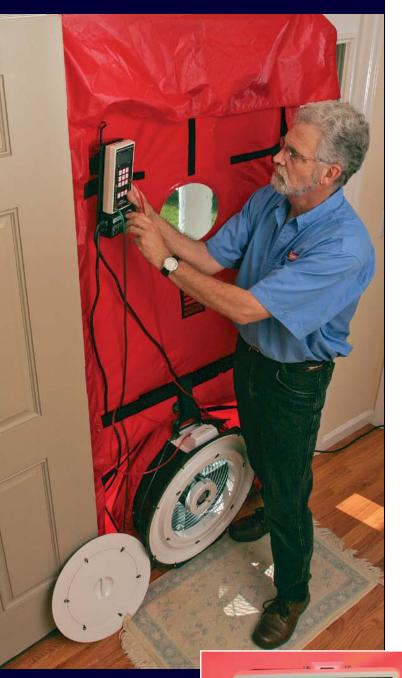
Start slowly. Gradually increase the fan speed with the controller until the manometer reaches about -25 Pa. Walk around the house to look for problems such as blowing fireplace ash or lifting vinyl flooring. If everything's OK, increase the speed to reach -50 Pa, then record the results.
