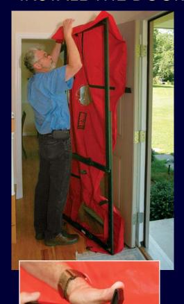
**Size and cover the frame.** Assemble and adjust the aluminum frame so that it's slightly loose in the opening but so that the cam locks will tighten the fit and lock the door in place when they're rotated. Remove the frame for installing the fabric cover.
