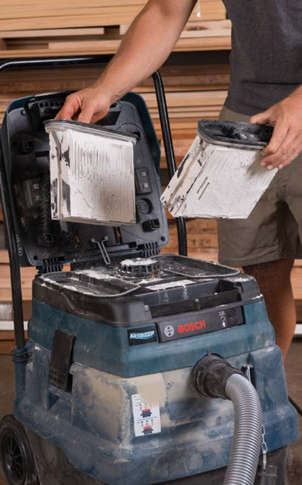
Cleans while you work. Available on a few of the top-brand vacs, self-cleaning filters mean the difference between poor suction from caked filters (left) and suction that stays strong.
