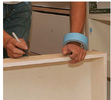
Drawers. Pullout shelves and drawers are labeled on the back side of the back panel to keep the marks hidden.
