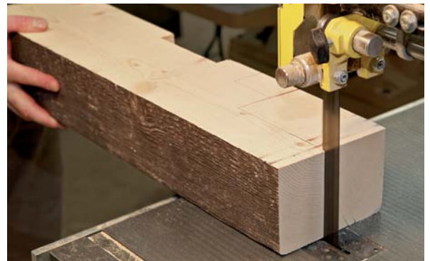
Fast cuts on thick stock. To cut the pillowed steps in the bracket post, first crosscut each step, then rip away the waste.
