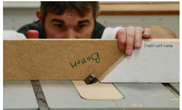
One-pass notch. After mitering both ends of the diagonal brace, notch the ends with a dado blade mounted in a tablesaw.
