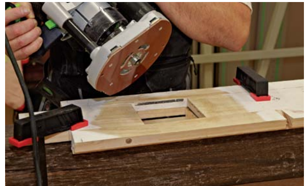
Router jig makes quick mortises. Used with a plunge router, this jig guides the cuts for the brace mortises. The workpiece is captured between adjustable stops, which can be repositioned for the longer vertical post.
