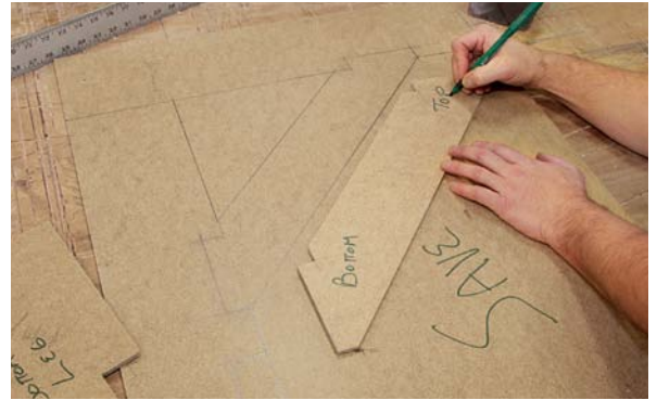
Retain consistency with templates. Draw each of the three parts of the bracket full scale on 1/4-in. hardboard, and cut it out as a template.
