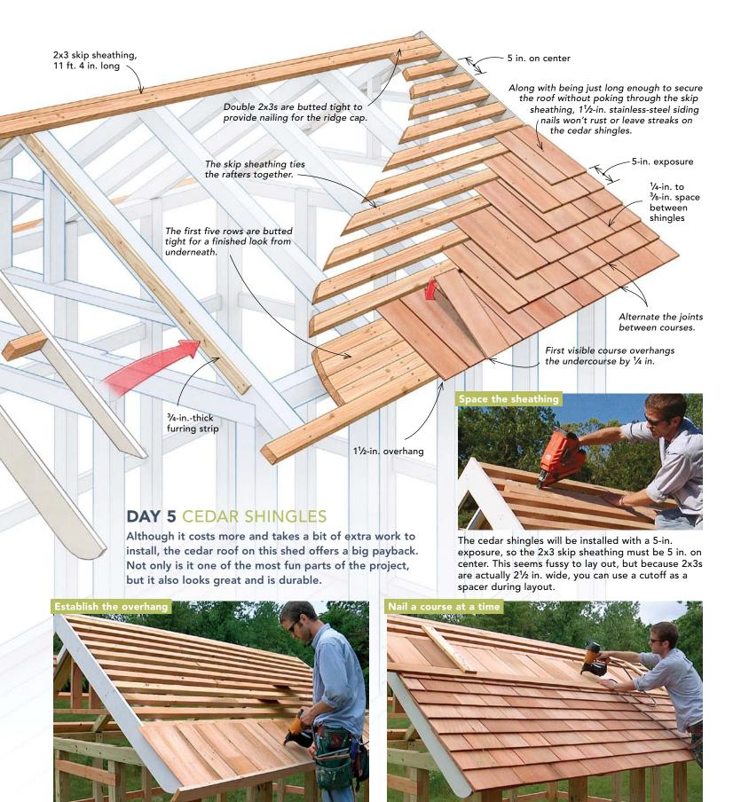
Tack a 2x4 spacer and ledger to the rafter tails to establish the 1½-in. overhang for the undercourse shingles. Once the undercourse shingles are in place, remove the spacer and ledger to make room for the first course of visible shingles, which will overhang the undercourse by an even ¼ in.
