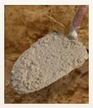
Too wet: Soupy concrete dilutes compressive strength. As the extra water dries away, tiny holes remain and weaken the concrete.
