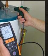
combustion analyzer also must have a nitrogen-oxide (NOx) filter; otherwise, the CO reading will be artificially elevated. Newer models include a NOx filter, and older models can use an add-on filter (\$40). The Testo 310 (shown here) has a NOx
