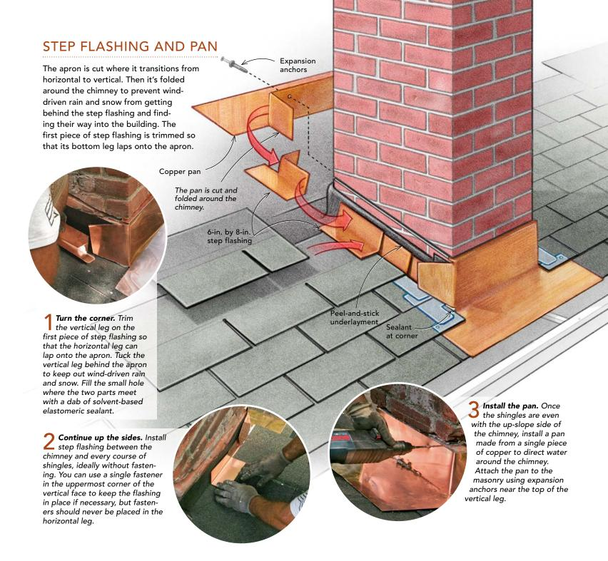
vertical legs are covered with counterflashing. The counterflashing directs falling rain and water running down the chimney over the first layer of flashing. This creates a finished assembly that looks good and, more important, is watertight.
