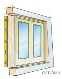
Hang the door plumb A door hung perfectly plumb in an out-of-plumb wall functions properly with little fuss, but the trim or extension jambs have to be altered. This is often the best choice for frequently used doors.
