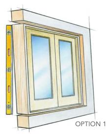
Hang the door in plane Hanging the door in plane with the wall often looks best because trim and extension jambs are uniform in width and thickness. Unfortunately, a door hung to match an out-of-plumb wall often swings open or closed on its own.
