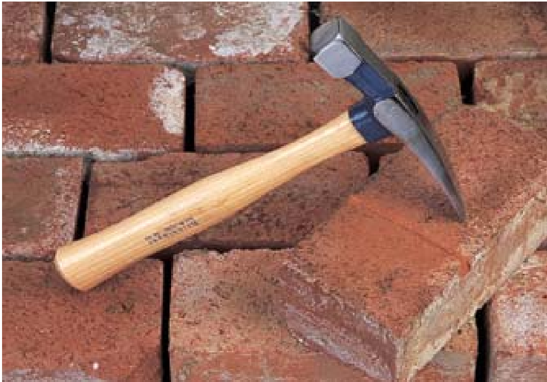
▲ BRICKLAYER'S HAMMER A bricklayer's hammer has a wide pick end for trimming bricks and a striking end for tapping bricks into position when they're set in mortar.
