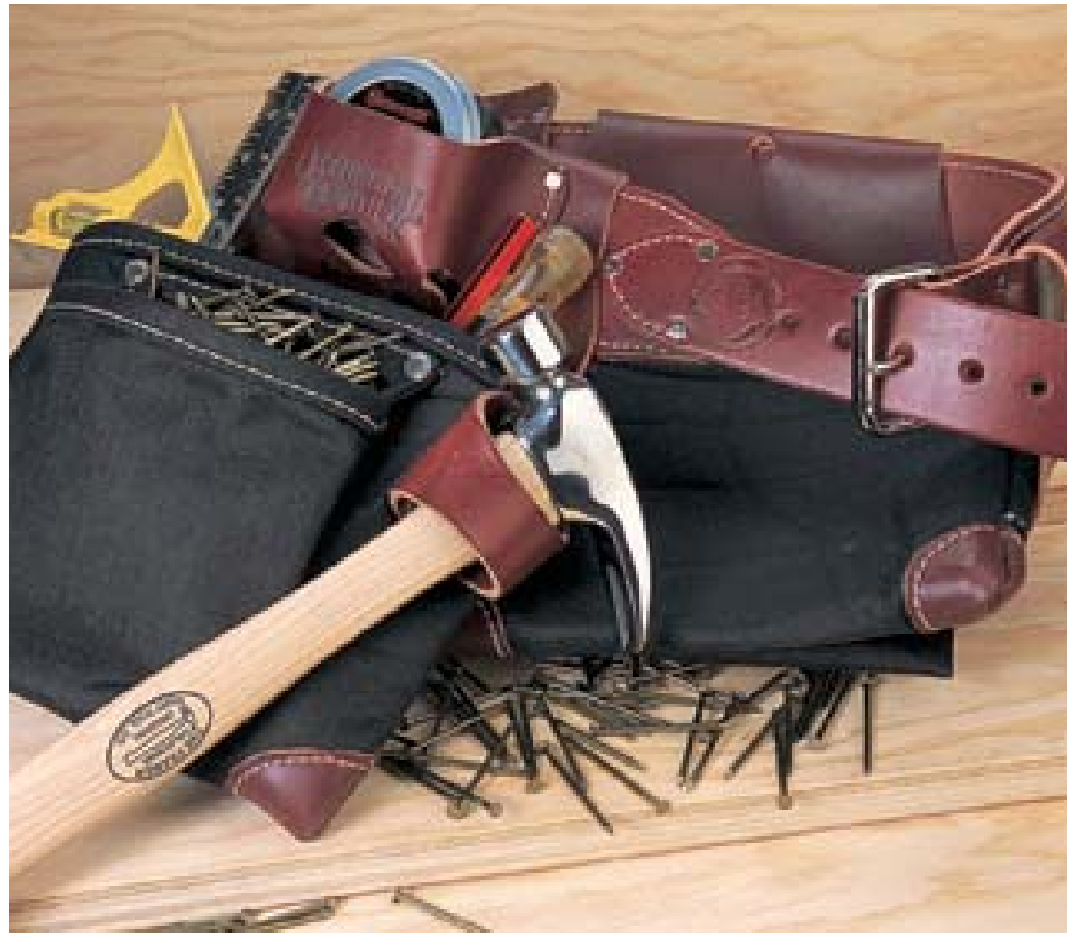
▲ CLAW HAMMER No carpenter's tool bag or kit is complete without a good claw hammer, indispensable for driving and pulling out nails, pounding and aligning parts, and even doing light demolition work.
