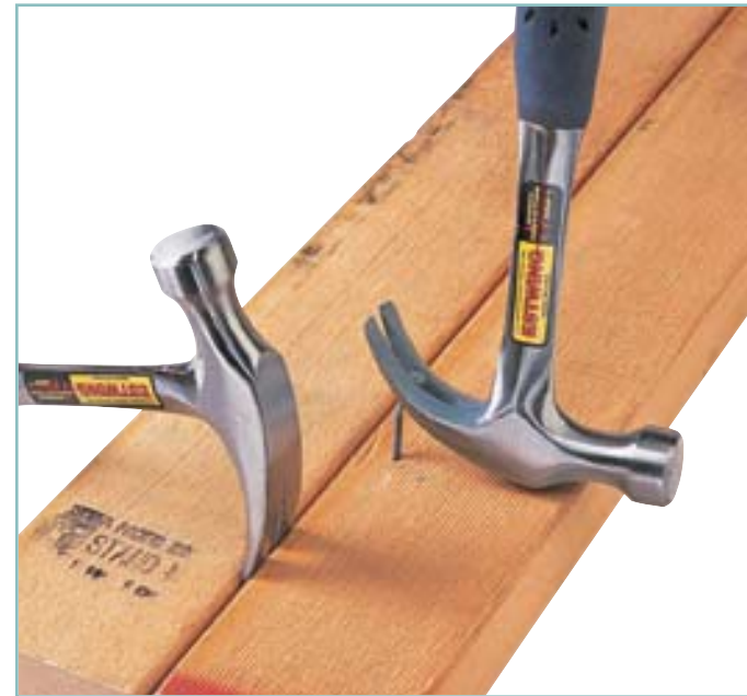
▲ CURVED-CLAW AND RIP-CLAW HAMMERS If you need a hammer with the leverage to pull out bent nails, choose a curved-claw model (right). Rip-claw hammers (left) can also pull out nails but are better for prying up boards or tearing up walls and floors.
