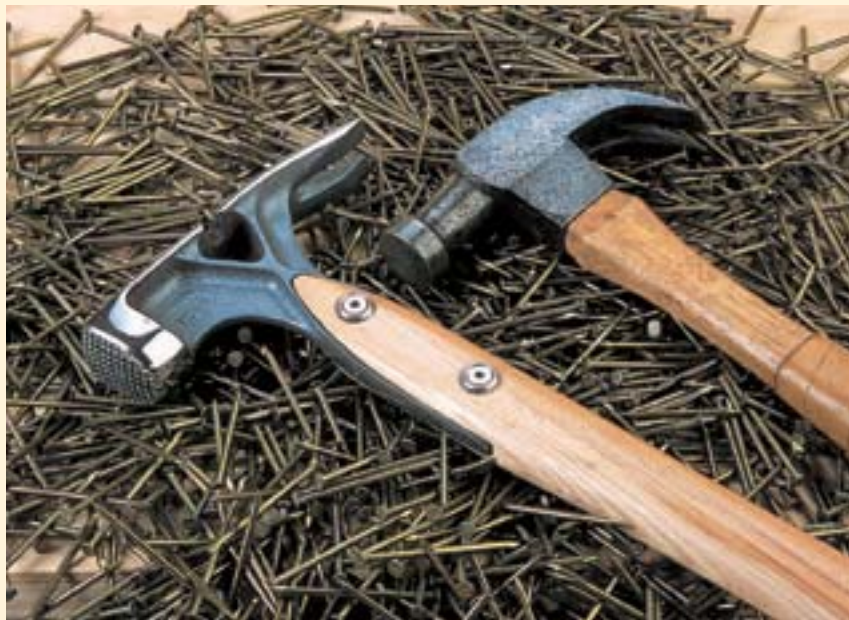
▲ HAMMER SIDE CLAW Long end claws found on most carpentry hammers are fine for pulling up large nails, but a side claw is handier for removing small nails and tacks.
