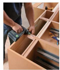
Fasten the blocking. Using 11/4-in. coarse-thread pocket-hole screws, fasten blocking between the top of the plywood and the adjacent cabinet backs. The blocking prevents the plywood panel from warping.
