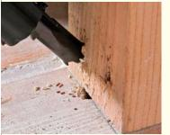
**▼ Toenailing spikes** that really grab are the key to fast, accurate toenailing. Look for a nose with especially sharp spikes protruding well out from the sides.
