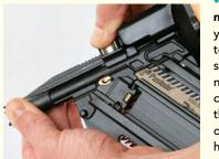
• A nonmarring nose cap allows your framing nailer to become a siding, trim, or deck nailer. Without a cap, the teeth on the nose turn cedar or redwood into hamburger.
