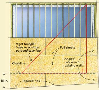
A right triangle is used to create a reference line perpendicular to the floor joists. The line should be 48 in. wide at its widest point to match the panel width.
