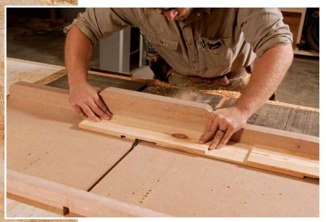
**Cut the dadoes.** The author milled the half-lap dadoes with a dado stack and a 4-ft.-wide crosscut sled, making sure to have plenty of room and support for the boards on each side. Each dado's orientation was marked on the edges, so he flipped the board back and forth as he went. It's easier to cut to the lines on each side of the dado and then to plow away the remainder.
