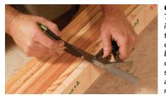
Gang the layout. The pole comes back into play for marking the flooring stock for dadoes. Clamp all the boards of the same orientation to the story pole, and use a combo square to mark off the layout.
