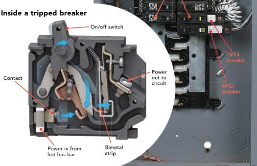
internal electromagnet will pull the electrical contacts apart.
