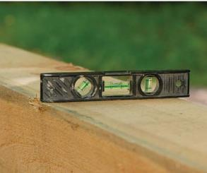
Find level. Because most timber-frame joints are made by drilling and cutting plumb, a level timber improves accuracy. While shimming the legs of the sawhorses is a possibility, the best option is to start with a level piece of ground or, even better, a shop floor.
