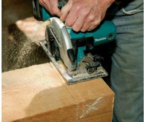
**Keep the cut shallow.** To compensate for out-of-square timbers, adjust the blade depth to the shallowest cut. Once the shoulder is cut, kerf out the remaining tenon waste.
