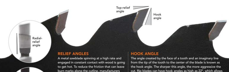
Tangentialrelief angle burn marks along the cutline, manufacturers angle the teeth of some sawblades to minimize the surface area that comes into contact with the wood and to provide space for dust and chips (and the heat they contain) to escape. The top-relief angle is generally 12° for softwood and 15° for hardwood. Slight radial-relief and tangential-relief angles help to prevent burning along the sides of the kerf, although they can produce scratch marks.
