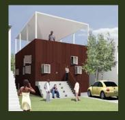
Architects were asked to design entries that connected the houses to the streetscape despite their elevation. Wide cast-in-place concrete steps with "stadium seating". shown in this design by London-based Adjaye Associates—provide one answer. The Adjaye design also features an inverted roof pitch to simplify rainwater collection.
