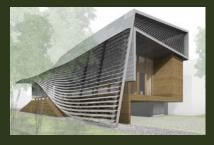
The roof of the house designed by Trahan Architects of New Orleans acts as a shading device, rain screen, solar-energy collector, and solar water heater. On the sloping side, the louvers, or "gills," are constructed to act as small gutters, channeling water into a retention system.
