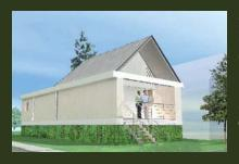
Shigeru Ban Architects of Tokyo based its design on a "structural furniture unit" intended to incorporate structure, storage, and insulation needs in a series of prefabricated units. The design is attributed in part to the observation, made in the aftermath of a Japanese earthquake, that the safest places in a house were under furniture or door frames. The model built by MIR was constructed with SIPs.
