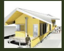
Only one MIR house was not built above base flood elevation—and that's because it was designed to float. Conceived by the architecture firm Morphosis and prefabricated by UCLA architecture students, the home's Saebi Alternative Building System (SABS) foundation is designed to function as a raft. The composite system consists of an expanded polystyrene core sprayed with reinforced concrete. The home's expense and its limited size, however, have made it impractical to replicate.
