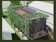
The house designed by Philadelphia-based Kiernan Timberlake Associates (photo p. 52) has a customizable floor plan built on a standard chassis that can be personalized further through details in the grillwork and the choice of a gable or garden roof.
