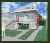
The single-family house designed by Billes Architecture of New Orleans has proved the most popular. In response to the local climate and drawing on traditional architectural elements, the home uses natural ventilation, high ceilings with fans, controlled daylighting, shading devices, and thermal mass to provide comfort with less reliance on mechanical systems.
