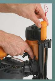
Quick cap reloads. The Bostitch tools use cylinders of caps that are held together by a plastic cord. After you've loaded the caps into the tool, just yank out the cord to free the caps.
