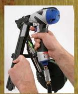
A twist of the wrist. Many of the staplers have the cap track and fastener track on opposite sides of the tool. Despite this larger look, these tools can still be turned to fit into tight corners fairly easily.
