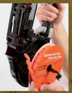
Free or cardboard coils? The Spotnails TCS6832 takes free-coiled caps, which are prone to unspooling if mishandled. The Duo-Fast and Paslode (shown here) use cardboard-sided coils that resist unspooling. If the coils get wet, the caps won't feed properly.
