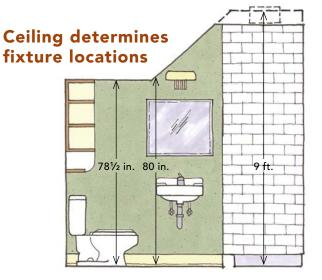
According to code, at least 50% of any room with a sloped ceiling must be at or above the minimum height of 84 in., and no portion may be below 5 ft. Code also specifies a minimum ceiling height of 80 in. over fixtures. The ceiling height below the stairs was just high enough to satisfy code with the minimum height at the front of the toilet.
