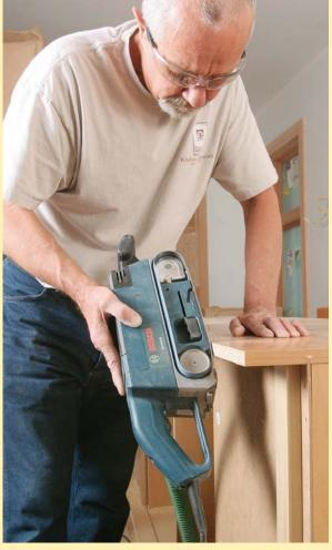
5 Bevel the edge. With a belt sander, remove the rest of the waste while giving the edge a bevel. Beveling the back of the panel ensures that the cabinet's outside edges will fit tight to the wall.
