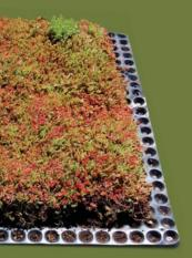
TILES Tiles are comprised of a base layer made of drainage material that is covered with a thin layer of soil and plants. Similar to modules in grid form, tiles can be installed quickly and provide instant visual appeal. While the work is fast, it still demands care, as improperly handled tiles can easily lead to loss of growth medium and plant damage. Tiles are best used on low-slope roofs. They can be used on steeper roofs, but above a 3-in-12 pitch, they demand a retention system.
