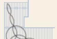
Start by overlaying the design on a deck plan with standard 12-in.on-center joist framing.
