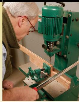
Dialing in the mortises. After the panel groove is cut, the mortiser is set up to cut on center and to the correct depth. Here, the mortises were cut to 15/16 in. deep to make room for glue and a 11/4-in.-long tenon.
