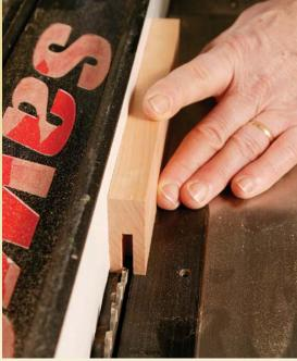
Two passes cut the panel groove. Although the groove is often cut with a dado stack, it also can be cut with a single tablesaw blade. Because the panel groove measures ¼ in. wide, it can be cut by positioning the fence so that the blade cuts just to one side of the centerline. Registered from either side of the stock, the blade cuts a centered groove in two passes.
