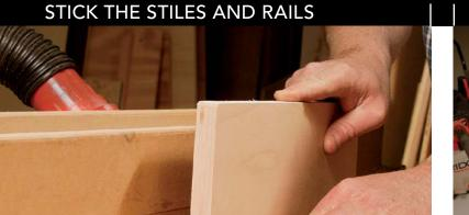
Switch to the stick bit. After switching bits, align the middle cutter with the stub tenon on the coped end. Run a test piece to make sure the mating cope and stick align. Run all rails and stiles.
