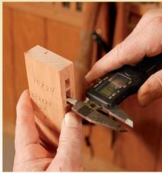
Make a test piece first for setup. The one fixed dimension of the mortise and tenon is determined by the size of the mortiser chisel, so the tenon and panel groove are sized to the mortise. A test mortise is cut with a benchtop mortiser fitted with a 1/4-in. bit. Measuring the width of the mortise with a set of dial calipers is an accurate way to determine the necessary thickness of the tenon and the panel groove.
