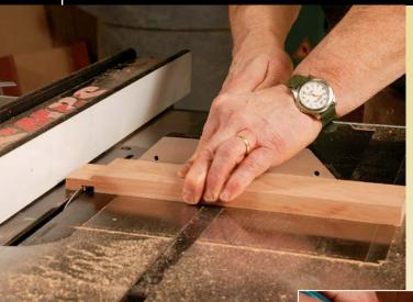
Tenons are crosscut on the tablesaw. Using either a single blade or a dado stack, tenons are cut by first registering the fence at a distance from the blade equal to the length of the tenon. The first pass will cut the cheeks, so it's important that the miter gauge be square to the blade. Moving the stock away from the fence and making repeated passes removes the waste. It's a good idea to check the setup on scrap first.
