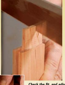
Check the fit, and adjust if needed. Each joint should be tested to ensure a tight fit before assembly. It's best if the tenon needs a few swipes with a plane to fit, rather than having to add a shim.
