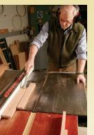
settings have been dialed in. For tooling, I use a tablesaw and a mortising machine in addition to a few basic hand tools. Mortises could be cut with a drill press or even a portable drill plus a chisel, but the mortising machine is faster and more accurate.
