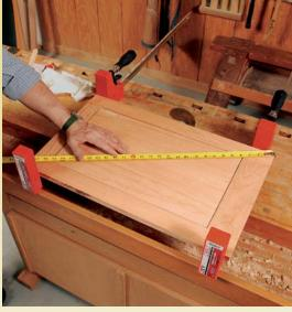
Cut and rabbet the panel. Once the frame is ready to be assembled, the panel can be cut. In this case, ½-in. plywood was chosen for a more substantial door. After the panel was cut to size, a rabbet was routed along its back edge.
