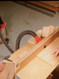
Prep the panel. Dry-fit the rails and stiles, then determine the panel size. Because plywood won't move seasonally, the panel can be cut within 1/16 in. of the actual size. The router table is set up with a straight or dado bit to cut the 1/4-in. by 1/2-in. rabbet on the back.
