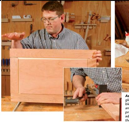
Assembly time. It's always a good idea to have a dry run when gluing up a door. If everything fits tightly, apply glue and assemble the rails, stiles, and panel. Clamp at both ends near the rails, and check that the door isn't curling because of too much clamp pressure. Parts that slide out of alignment under pressure can be adjusted back into place with a dead-blow mallet. Finally, check the diagonals to make sure the door is square.
