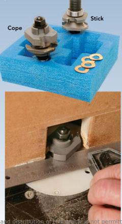
A two-bit approach. Copeand-stick router bits are available as single arbors with interchangeable cutters or in sets of dedicated cope and stick bits. The two-bit sets are more accurate and take much less time to set up. (The Amana set used here costs about \$120 and also can be used to make interior passage doors.) Many sets include thin brass or steel shims that can be inserted between the cutters to match the relative size of the profile to the thickness of the stock.
