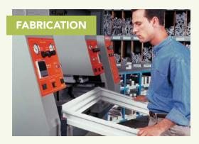
While the largest manufacturers may make their own profiles, many buy profiles from extruders. These long extrusions are then cut to size and joined together to make sashes and frames (photo above).
