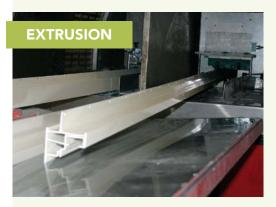
Vinyl extrusions (also known as profiles or lineals) are made by forcing hot PVC compound through a die. The resulting extrusion is a long, rail-like piece of plastic that includes webs and voids to provide rigidity (photo left).
