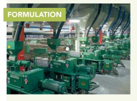
Manufacturing begins with the formulation of the plastic compound used to make vinyl extrusions. The compound consists of 80% to 85% PVC pellets mixed with 15% to 20% other ingredients, including heat stabilizers such as organo-tin mercaptides and a pigment (usually titanium dioxide) that helps to protect the vinyl from the harmful effects of UV-light (photo below).
