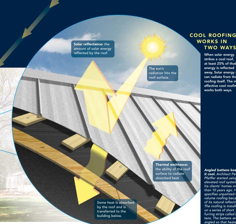
When solar energy strikes a cool roof, at least 25% of that energy is reflected away. Solar energy also can radiate from the roofing itself. The most
