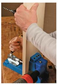
down and twisted to lock the stock into position. For subsequent pieces of the same thickness, you can quickly clamp and
