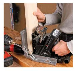
Kreg jig slides up and down, and is secured with a setscrew. On the Porter-Cable model, there is no depth adjustment to worry about. The collar on the drill bit pushes down on a metal plate, and the plate stops automatically based on the wood's thickness.
