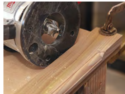
Routed embellishment. Clamp the sash stock securely to the work surface, leaving the stock long enough for the router to avoid bumping into the clamps at each end. Rout a 3/8-in.-radius quarter-round thumbnail profile along the inside front edge of the outside sash stock.
