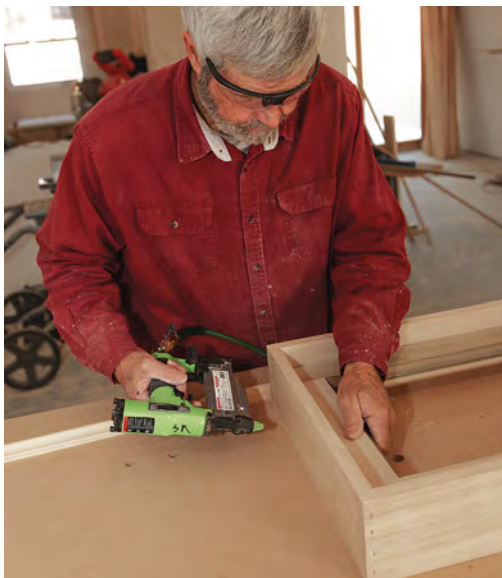
Second stop holds the sash. With the jamb square and the sash tacked in place, apply the inside bead of sash stop to permanently secure the sash in the jamb.
