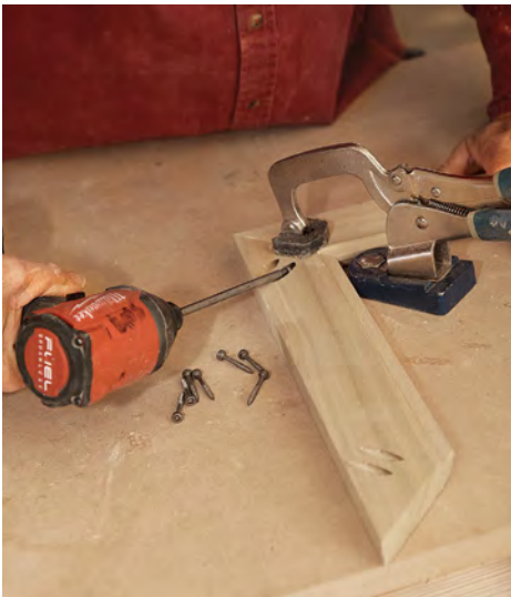
Pocket-screw assembly. After drilling pocket-screw holes in the shorter vertical pieces, drive headless pins to keep the corners aligned, then secure the corners with pocket screws.
