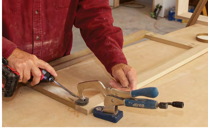
Butt joints for the back side. The frame for the back side is planed to 2 in., which leaves space for the glass between the frames. Butt joints are an easier way to build the back half of the sash, but pocket screws still make the strongest joints.
