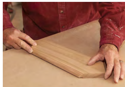
Tight miter secret. To get tight mitered joints, you have to cut the height and width pieces accurately. After cutting the miter angles on each pair, line up the long edges side by side to make sure they are exactly the same length.
