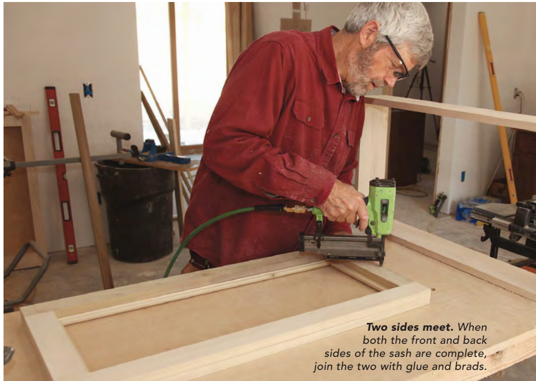
Butt joints for the back side. The frame for the back side is planed to 2 in., which leaves space for the glass between the frames. Butt joints are an easier way to build the back half of the sash, but pocket screws still make the strongest joints.
