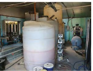
Special sauce. Admixtures like calcium chloride are dispensed by hand and added to the mix at the plant or on-site, depending on the additive.
