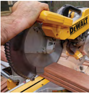
Gang cut. Measure the width of each stair and add 2 in. for a 1-in. overhang at both ends. Cut all pieces for one tread at once for accuracy.
