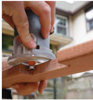
Round over the edges. All cut edges are trimmed with a 1/8-in. roundover bit for an eased profile that matches the one from the sawmill.
