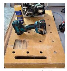
Customized tops. I've refined the carts a bit since initially building them. The tops especially are a great place for dog holes for workholding and assembly. A slot for a circular saw, a hole for a drill, and a recess for screws and hardware are all on my main assembly cart.
