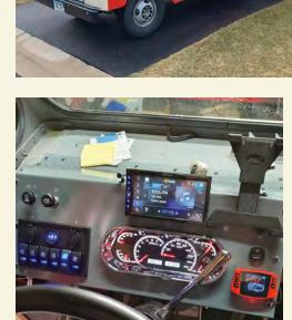
components were refurbished or rebuilt. The transmission was rebuilt, the rear end cleaned up, and the already rebuilt steering box reused, along with the frame and body. Suspension, engine, wiring, steering column, instruments, wheels, tires, radiator, power steering, and brakes are all new. The power plant is an HT383 "stroker" crate motor with 323 hp and 444 lb. of torque. When new, the truck's stock GM 350 produced 190 hp.
