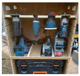
Efficiency in progress. The early tool holders were upside-down tees screwed to the cart top. Later I found that plywood with slots, set at an angle, makes getting tools in and out easier and keeps tools from falling out of the carts when in motion.
