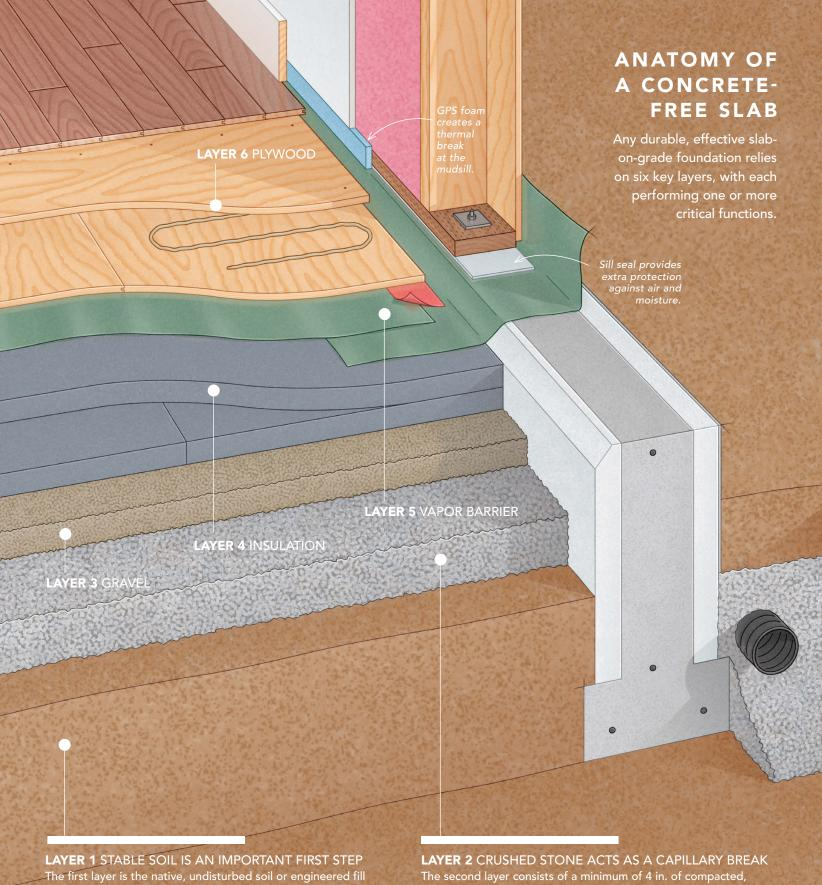
The first layer is the native, undisturbed soil or engineered fill that the slab, its footings, and ultimately the building bear on. Since we designed the building featured here to have no interior point loads, all the bearing is on the perimeter stem wall and footings, and the slab has no structural function. When we have a building with point loads or load-bearing walls on the interior, we add interior footings, just as we would with a concrete slab.
