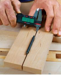
DIAL IN YOUR HINGE-MORTISING JIG Mortise two test pieces, equal in size to a door stile and a face-frame stile, to test the mortise depth and ensure a precise gap on the hinge side of the door.
