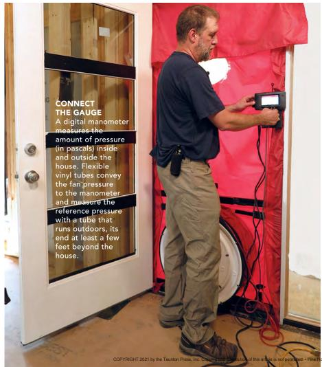
eter to my phone, which is now my preferred way to conduct most tests. I choose the exterior door where I'll install the blower door based on wind speed and direction. Wind can have a large effect on the test result, and the blower door should be on the leeward side of the building when winds are greater than 5 mph.
