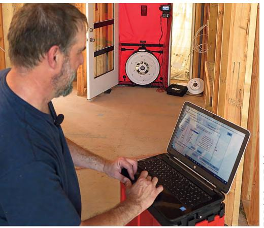
the cumulative area of air leaks in the shape of a smooth hole. Basically, this gives us an idea of how big a hole is in the building's shell at a natural building pressure. This is a handy visual for homeowners.
