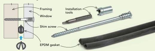
lag screw. A special installation tool grabs both parts simultaneously so that the screw can be installed in a hole drilled in the window frame. The tool is then used to screw the lag into the rough framing while the sleeve remains fixed in the window frame. Then the lag screw can be adjusted to make the window plumb and level.
