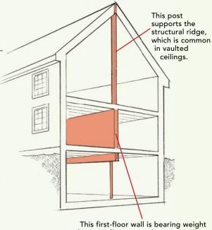
from the floor joists above, as well as the roof load. Bearing walls often run inline with a beam in the basement. They can be offset from their bearing points, however.
