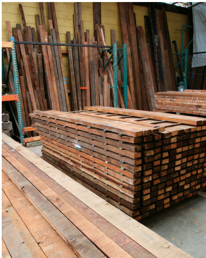
Old forests reclaimed. This big stack of old-growth-fir studs came from the house in southwest Portland featured in this article. Salvage Works kiln-dries every piece of reclaimed lumber it sells, and has a big bandsaw that can skim off lead paint.
