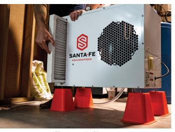
**Protective filtration.** The filter on a consumergrade dehumidifier is meant to keep the evaporator coil from clogging with dust or pet hair, not to improve indoor-air quality. But high-capacity units can have high-performance air filters that protect the equipment and clean the dehumidified air. This Sante Fe model has a 2-in. thick, MERV-13 filter.
