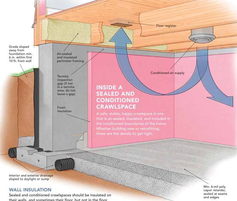
Sealed and conditioned crawlspaces should be insulated on their walls, and sometimes their floor, but not in the floor framing. Choose an insulation that isn't sensitive to water and effectively blocks the flow of air to prevent humid crawlspace air from coming into contact with the cool concrete surfaces.
