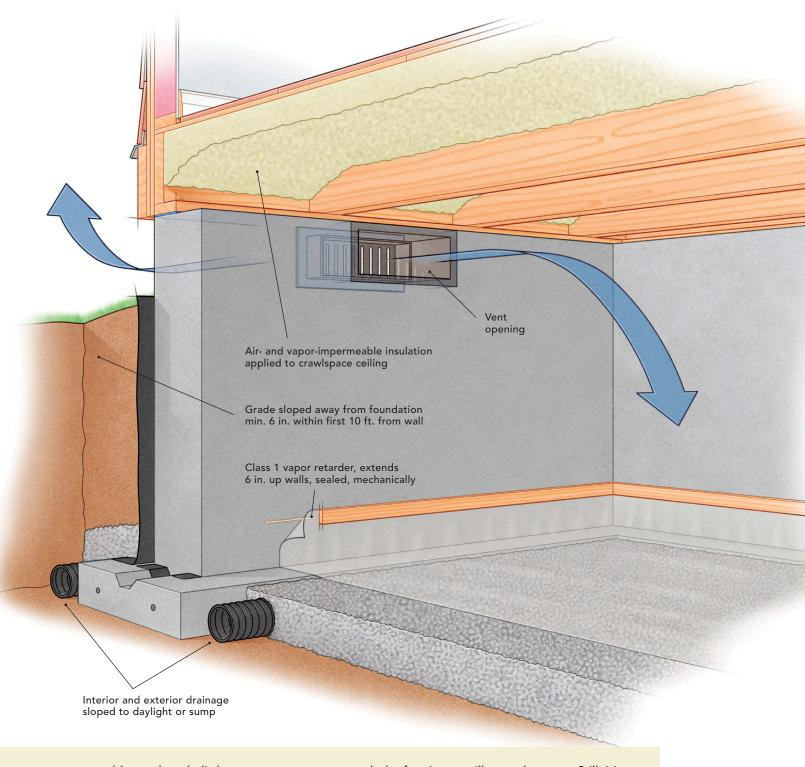
vapor permeable, so they do little to prevent humid crawlspace air from reaching the relatively cool framing lumber and sheathing of the floor. Moisture content in the lumber climbs, has little opportunity for drying—especially if the interior flooring is vapor impermeable—and rot sets in.
