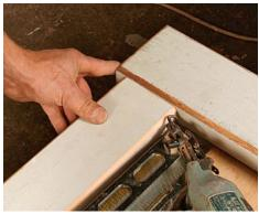
Toenail the corners. Place a toenail in the inside edge of the leg using 2½-in. galvanized finish nails. This adds strength to the joint while the glue dries so that it doesn't twist during the rest of the assembly.
