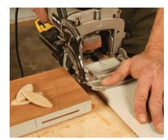
1 Slot the legs and the head. When the head and legs are different thicknesses, register the fence to the back of the stock. Register off the face when joining heads and legs of the same thickness.
