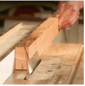
Straight stock gets an angled rip. Start with an appropriate length of 2½-in. by 1¾-in. stock. Rip a 15° bevel to create the sill's pitched face. Lower the blade and reset the fence. Then kerf the bottom of the sill to create a drip edge.
