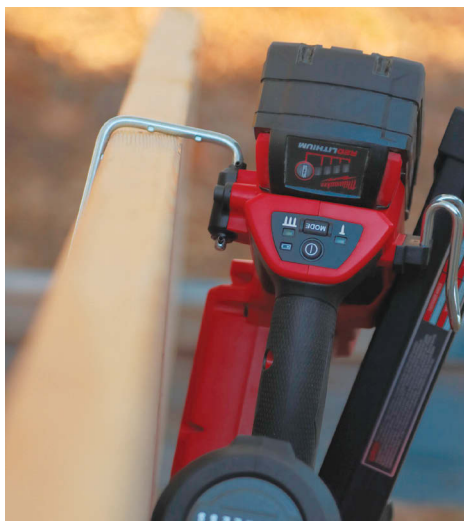
Just right. If the DeWalt rafter hook is too small, and the Metabo's is too large, Milwaukee's feels just right. These also include a belt loop, which the others omit.
