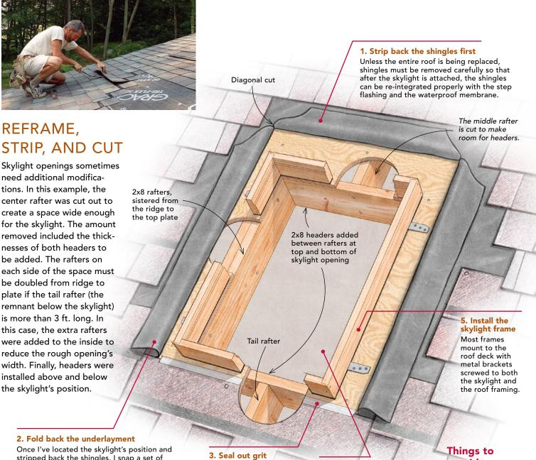
Once I've located the skylight's position and stripped back the shingles, I snap a set of chalklines on the roofing underlayment and remove that section. Next, I make 3-in.-long horizontal cuts at the bottom and 6-in.-long diagonal cuts at the top that splay out about 3 in. Then I fold away the underlayment flaps. I integrate these flaps into the flashing later.
