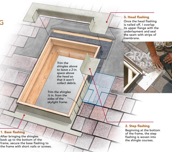
peel-and-stick membrane as the final line of defense against leaks. Applied meticulously around the skylight frame, the membrane collects water that gets beneath the metal flashing and redirects it to the shingle surface below the skylight.
