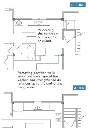
Reconfiguring the stair allowed for continuous cabinetry in the kitchen, plus a view down into the space from the second floor.
