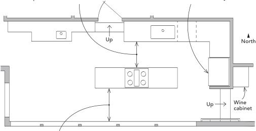
**THE THOROUGHFARE** has no seating and measures 42 in. from countertop to wall, which is narrow, but because there are windows on one side and an open island on the other, it gives the impression of more width.
