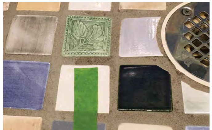
Green tape moved to expose the strip of grout that did not get any treatment. The Soft Scrub area is more clear of discoloration.
