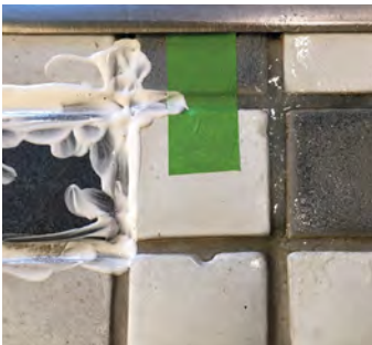
Cleaners applied: Soft Scrub to the left of the green tape and OxiClean to the right.
